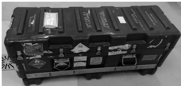
Fig. 2. Transport container for hydrazine gas cylinder
