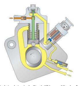
Fig. 5. Fuel circulation in the Bosch CP4 pump [Gunther 2014]
