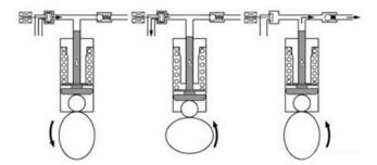
Fig. 4. Diagram of the operation of a section with a direct-action valve [Kedzia]
