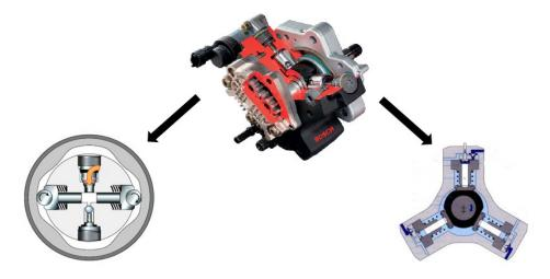
Fig. 2. Classification of common-rail pumps [Meyer 2003]
