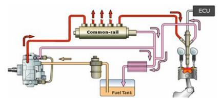
Fig. 1. Diagram of a common-rail system [Gunther 2014]
