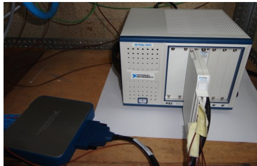
Fig. 16. NI PXIe-1073 control platform with NI PXIe-6341 and NI TB-4353 cards
